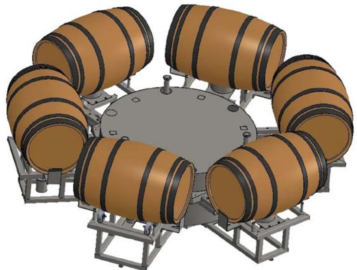
■ Several barrels washed at the same time, continuous washing when barrels are loaded one after another.
