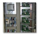
Vinicontrol is an electronic regulator capable of managing two outputs with two independent settings. Designed around an electronic board developed in house, it comes in a watertight case ( **CE** standard) with outputs and inputs (probes) on a plugin connector.
